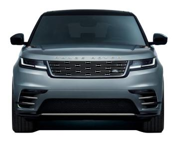
Maximum height 1.678mm (Air) 1.683mm (Coil)
